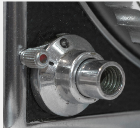
Time mode. Release button will be locked in the in-position.
